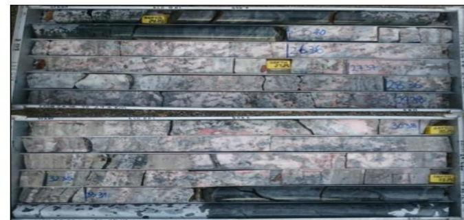
Typical Zoned Pegmatite in ACD001 showing pink and grey spodumene and petalite lithium minerals (above) and Arcadia cross section (left)
