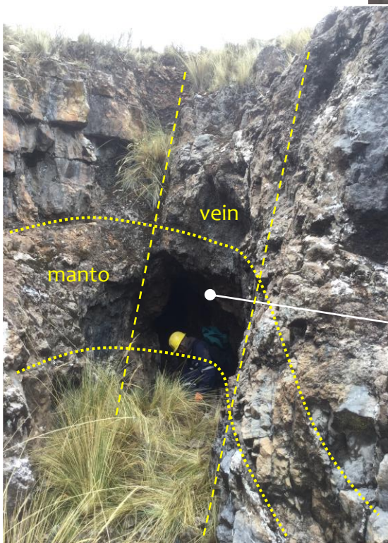
Figure 3: ABOVE A small mine working sampled during Program 4. The working is located at an intersection between a flat lying manto horizon (dotted yellow lines) and a sub-vertical vein (dashed yellow lines). RIGHT An old mine working exposing a flat lying 75cm to 100cm thick manto horizon sampled during Program 4.
