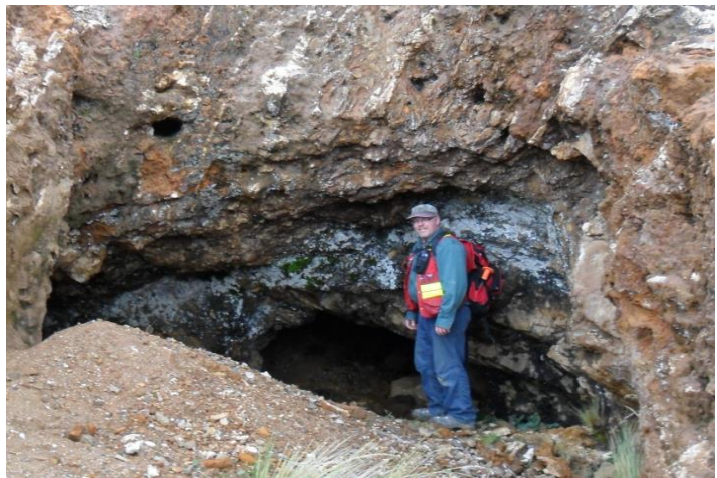
Old mine working at vein & manto intersection
