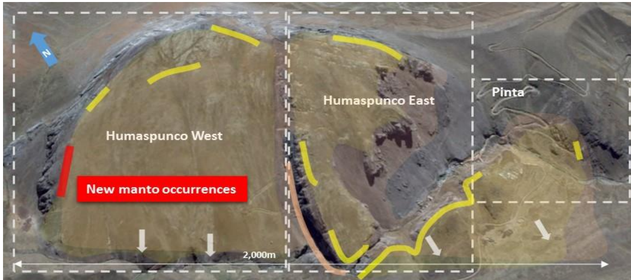
Figure 4: ABOVE Manto occurrences of Humaspunco-Pinta. Previously known mantos are shown with yellow and orange lines. The approximate location of the new upper manto horizon occurrence is shown in red. Mapping now shows that manto mineralisation occurs around much of the perimeter of Humaspunco Hill. It also occurs as an outlier at Pinta and as inliers along the central Humaspunco ridge. The known manto sequence is now relatively well defined by the limits of Humaspunco Hill. As previously described, the manto sequence dips into the ground to the south, where it is open (at depth). Repeat mantos (in the same horizontal plane) are possible at depth.
