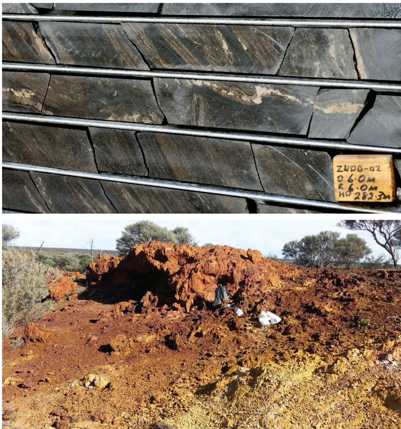
Figure 4.2: Drill core ZNDD02 (top) showing intersected mineralisation and gossan surface expression of mineralisation (bottom) (Heron Resources)
