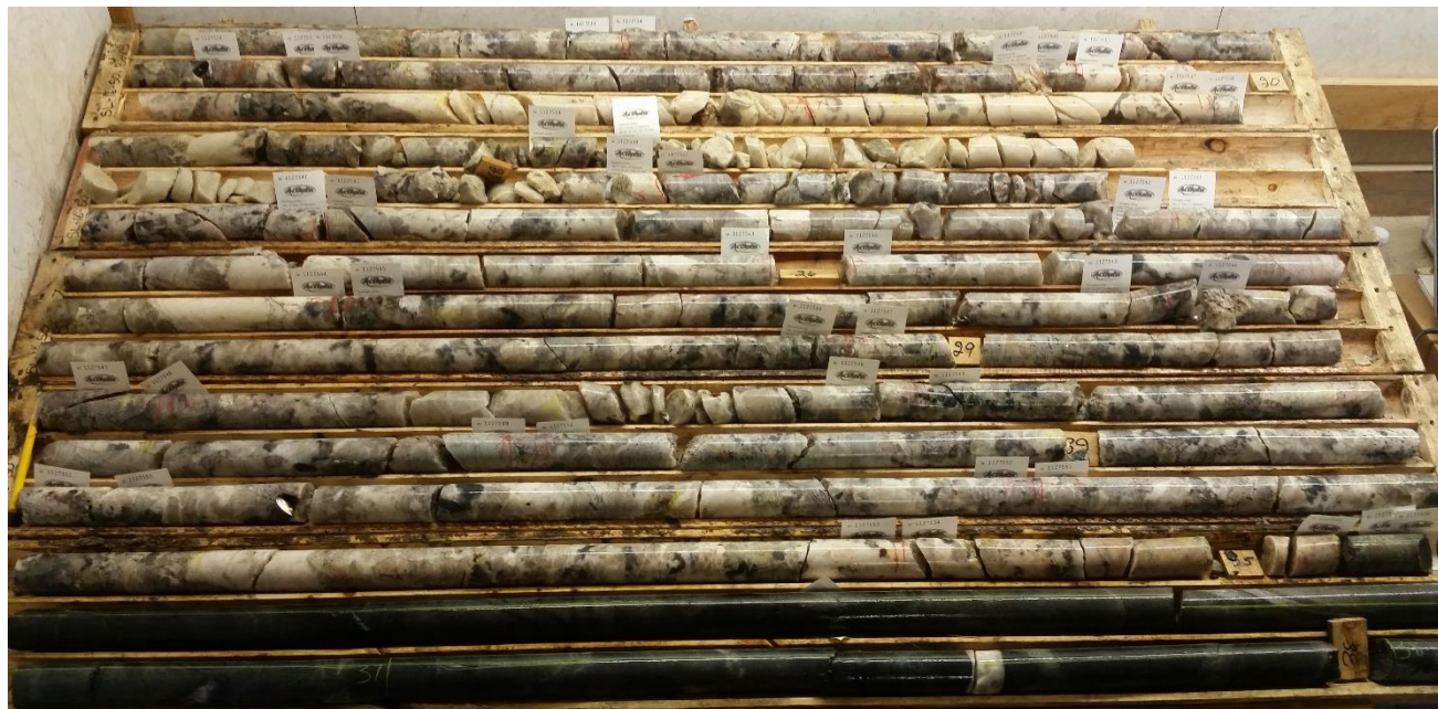
Figure 2. Drill core obtained from hole SL-16-50 showing an intersection of 18.23m of spodumene-bearing pegmatite.
