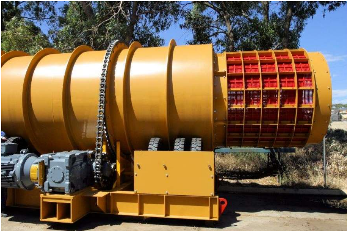
↑ Attrition scrubber of the type that could be used for a saprolite-hosted graphite operation
