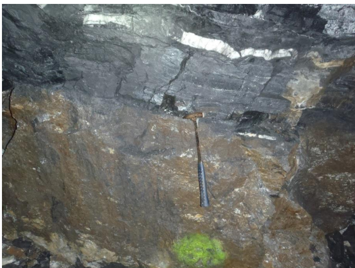
Figure 2. Massive sulphide mineralisation on Level 8 showing sheared upper contact with shales
