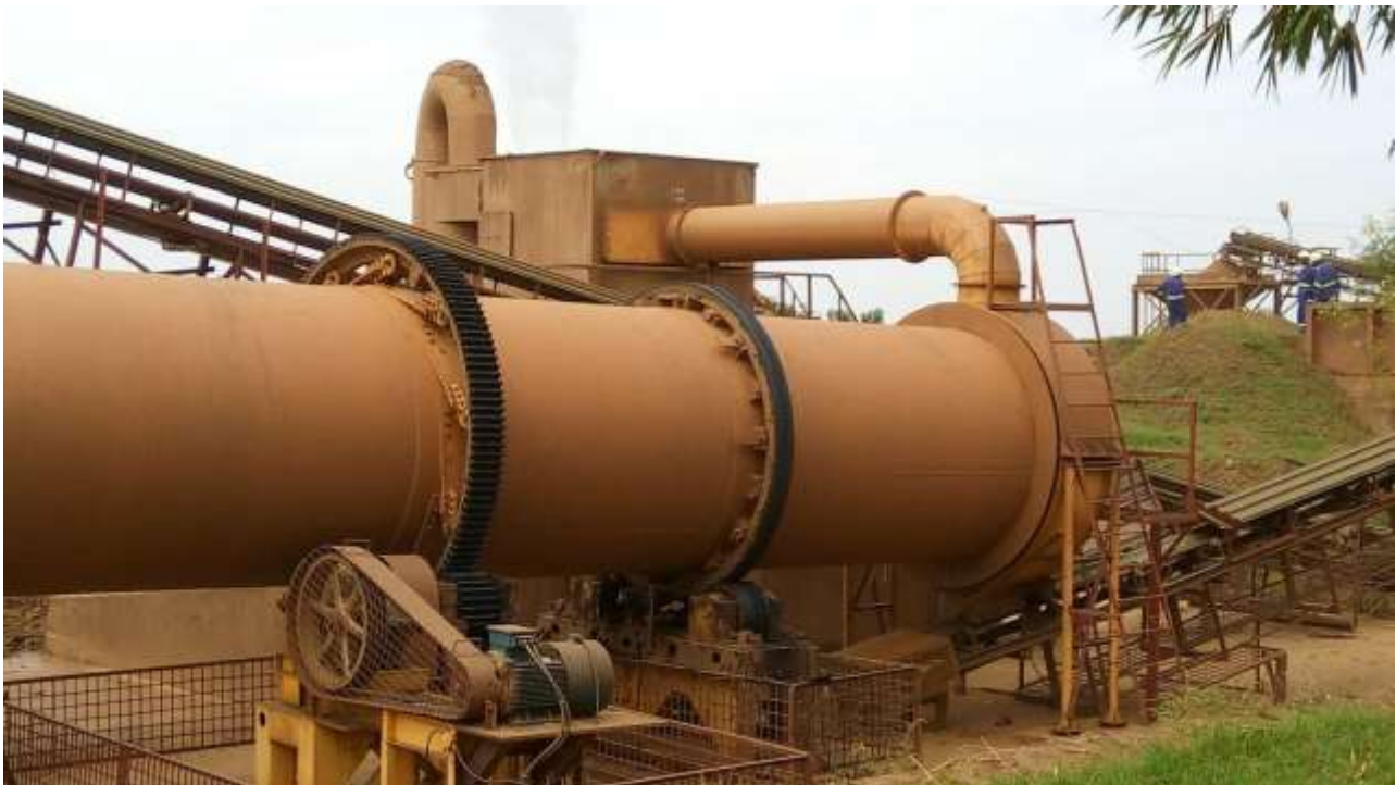
Vermiculite is then fed into the rotary dryer to lower the moisture content - November 2016
