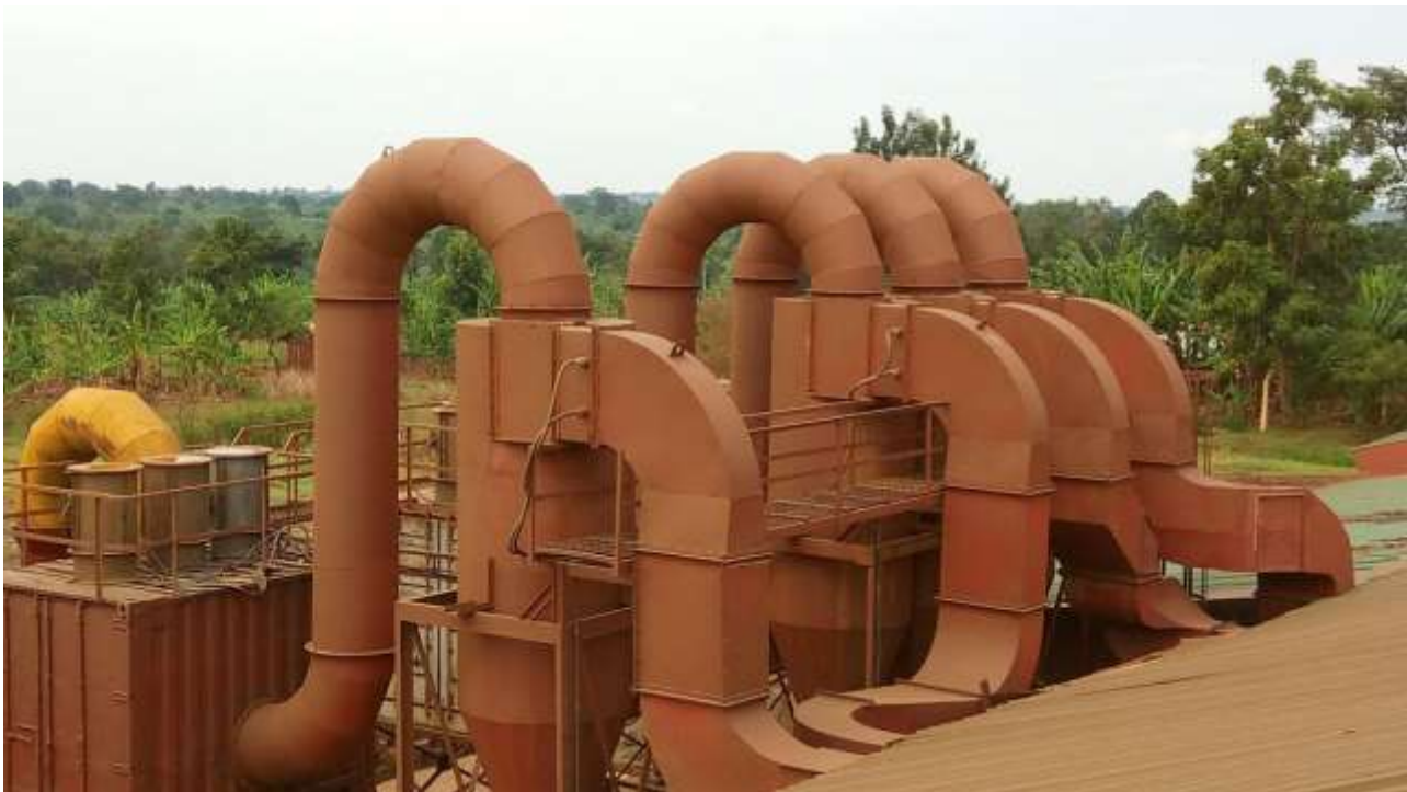
The separated, different sized ore fractions are then passed through winnowers - November 2016
