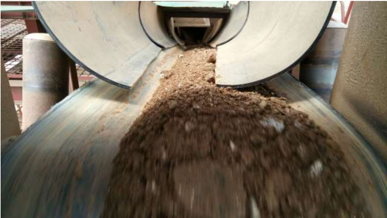
Vermiculite from ROM Bin conveyed to the magnetic separator - November 2016
