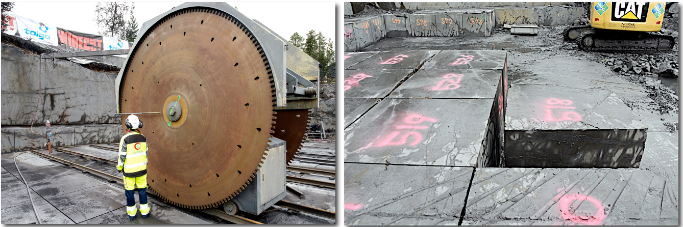
Figure 2 Ore block cutting (L) and extraction (R) at Talga's Vittangi graphite project trial mine, Sweden.
