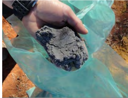
Sulphide rich RC sample in RCLR161
