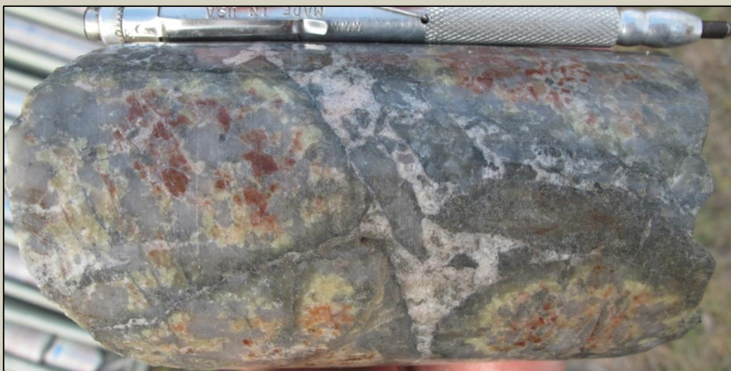
Breccia with white (?calcite) and pink (rhodochrosite) carbonate and pyrite infill at 222.5m
