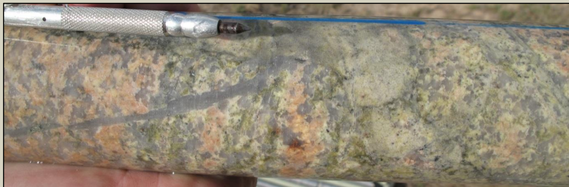
Polymictic breccia with epidote sericite alteration at 234.5m
