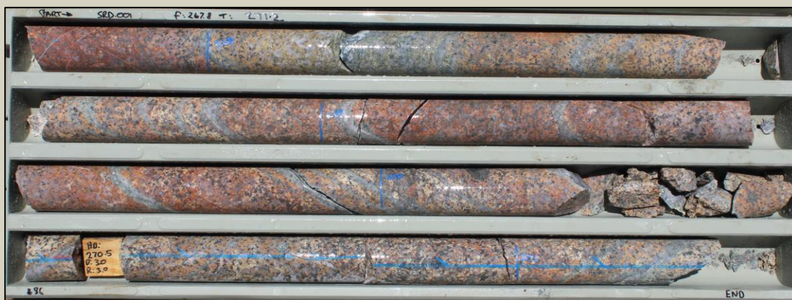
Sheeted quartz-pyrite veins in red rock altered Barrabas Adamellite at 270m
