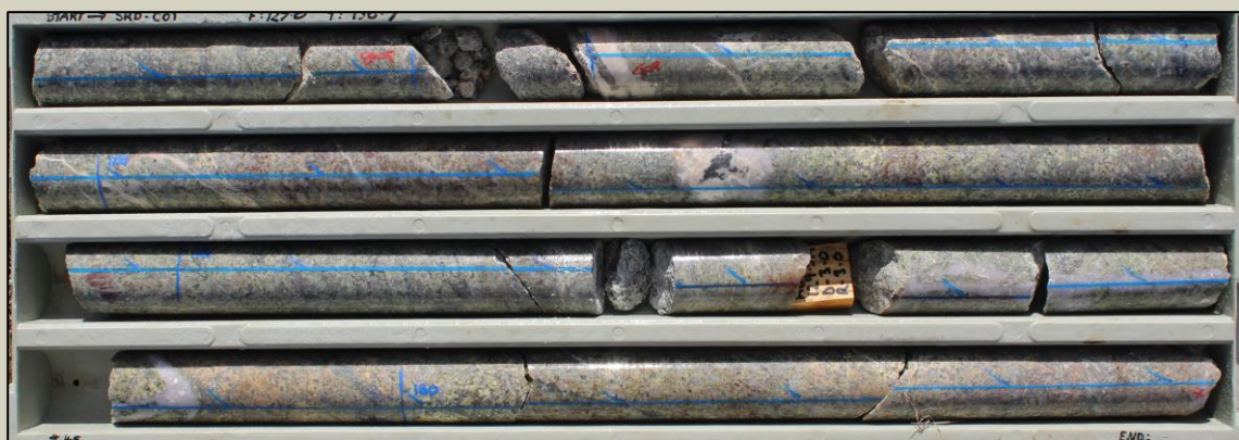
Variably altered breccia with quartz veining at 128m
