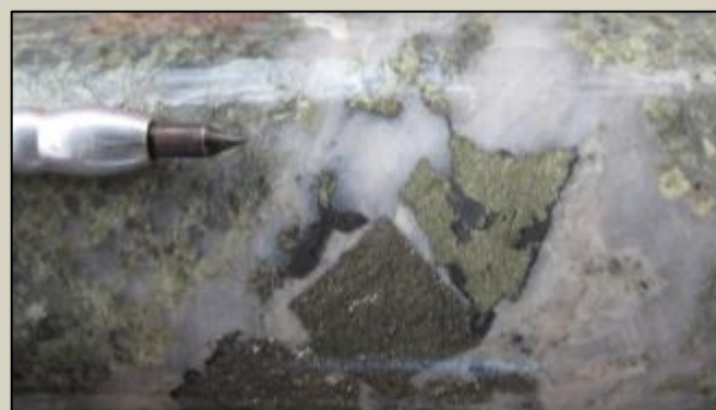
Pyrite-chalcopyrite-tennantite-tetrahedrite in a quartz vein at 128m
