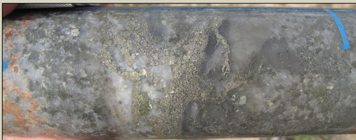
Pyrite-chalcopyrite veining/breccia infill in chlorite-sericite altered breccia at 225m
