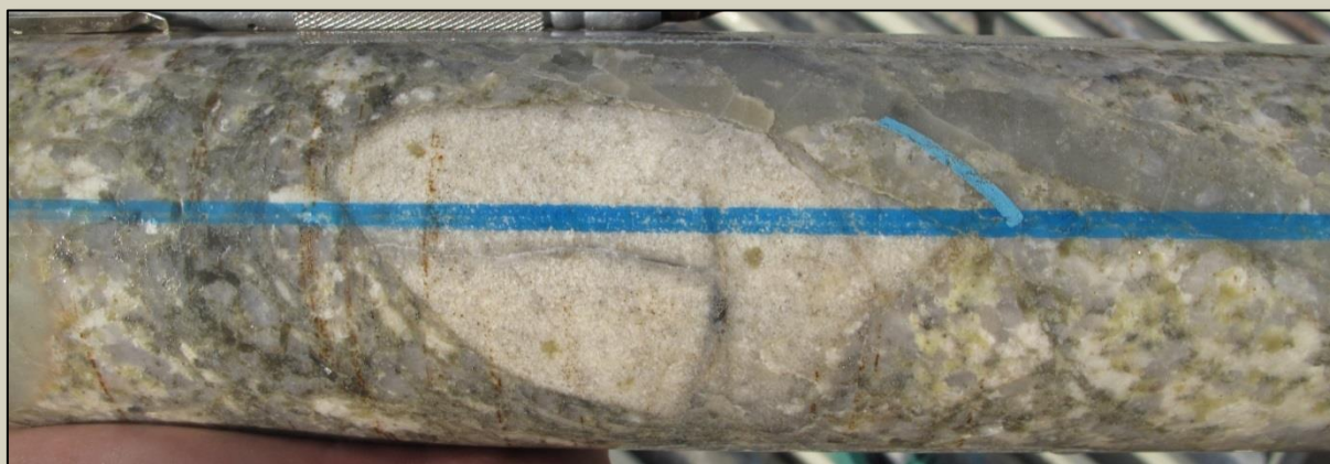
Sericite altered aplite clast in sericite-?silica altered breccia at 156m
