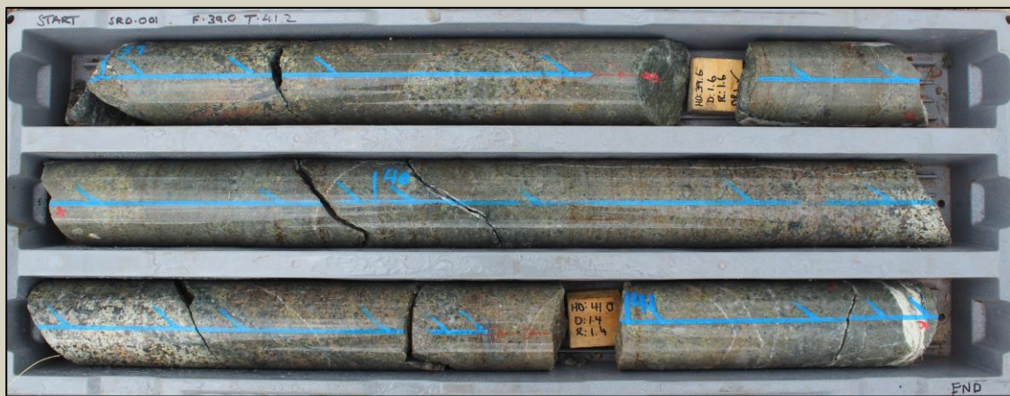
Altered breccia with clasts of altered Barrabas Adamellite at 40m
