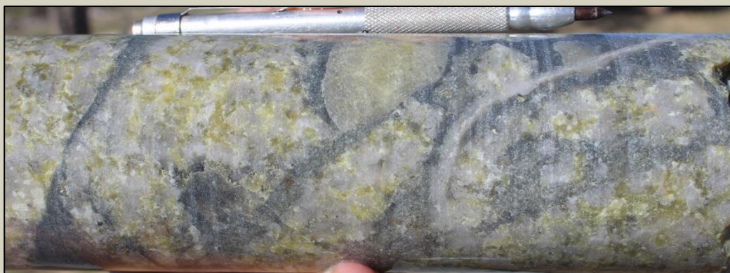
Clast supported breccia with sericite alteration within clasts at 131m – note the late quartz vein traversing both the breccia clasts and matrix.
