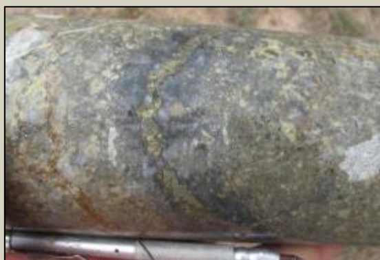
Quartz-pyrite-chalcopyrite vein with sericite alteration selvage
