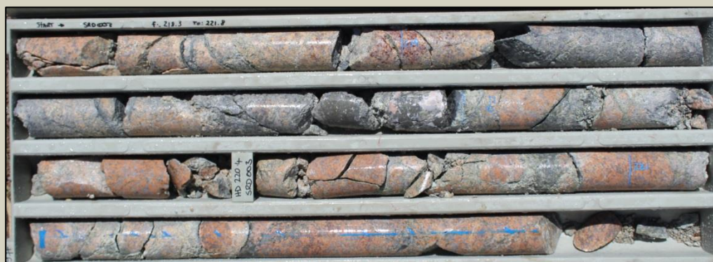
Fault zone at 219m to 221m
