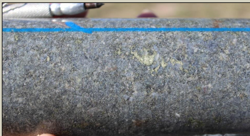
Matrix supported breccia with disseminated chalcopyrite-pyrite+tennantite-tetrahedrite at 120m
