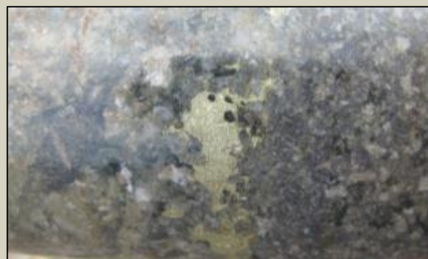
Chalcopyrite and molybdenite in breccia at 38m
