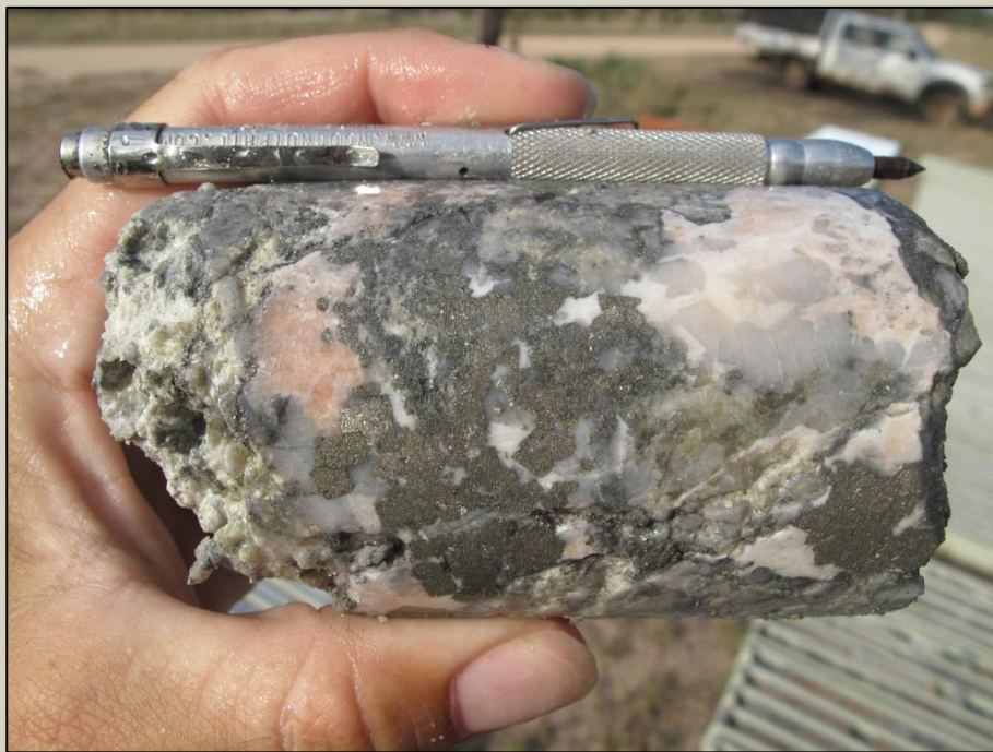
Pyrite-quartz-rhodocrosite-carbonate ± tennantite-tetrahedrite vein at 221m
