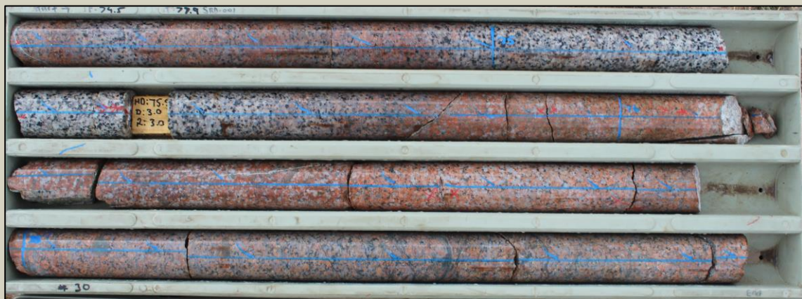
Weak to moderate red rock alteration of Barrabas Adamellite at 76m
