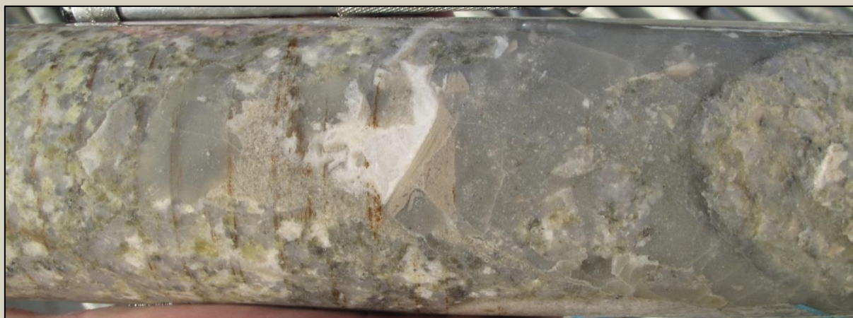
Chalcedonic quartz vein in sericite altered breccia at 156m
