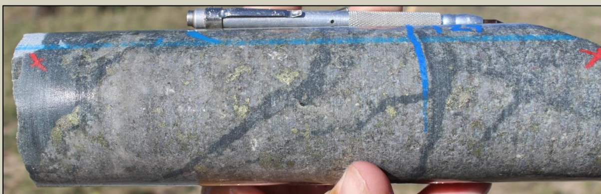
Clast supported breccia with increased percentage of chalcopyrite-pyrite+tennantite-tetrahedrite at 129m
