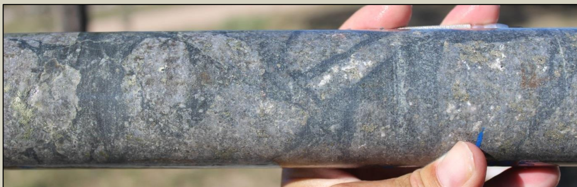
Clast supported breccia with chalcopyrite-pyrite mineralisation at 125m
