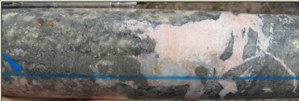
Breccia with rhodocrosite-pyrite-quartz in-fill at 222.3m
