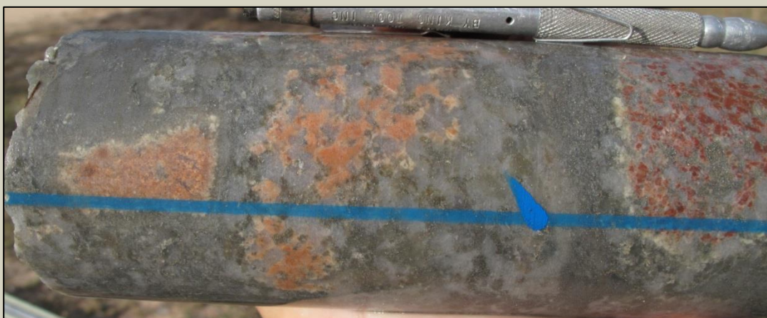
Clasts of adamellite in a strongly chlorite-sericite altered matrix. Clasts display alteration rims. 224.5m
