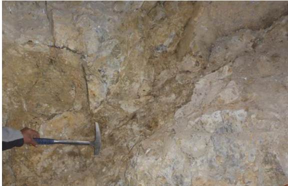
Figure 2: ABOVE LEFT Wall rock photo inside the Vilcapuquio mine working (upper level) showing a broad zone of highly altered stockwork veining (brown discolouration). ABOVE RIGHT Photo of a rock sample taken from this section of the mine.
