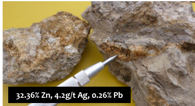
Figure 3: ABOVE LEFT Close-up of wall rock photo inside the Vilcapuquio mine working (upper level) showing stockwork veining (cream coloured lines) in less altered limestone (dark grey colouring). ABOVE RIGHT Photo of a rock sample taken from this section of the mine.
