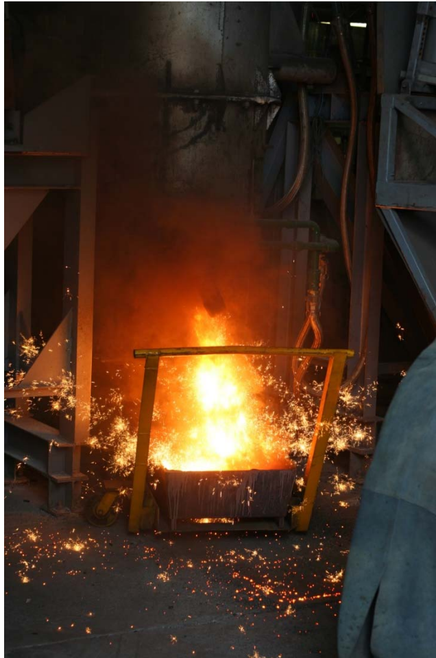
Ausiron process pilot scale hot metal tapping utilising Kulon Progo DRI
