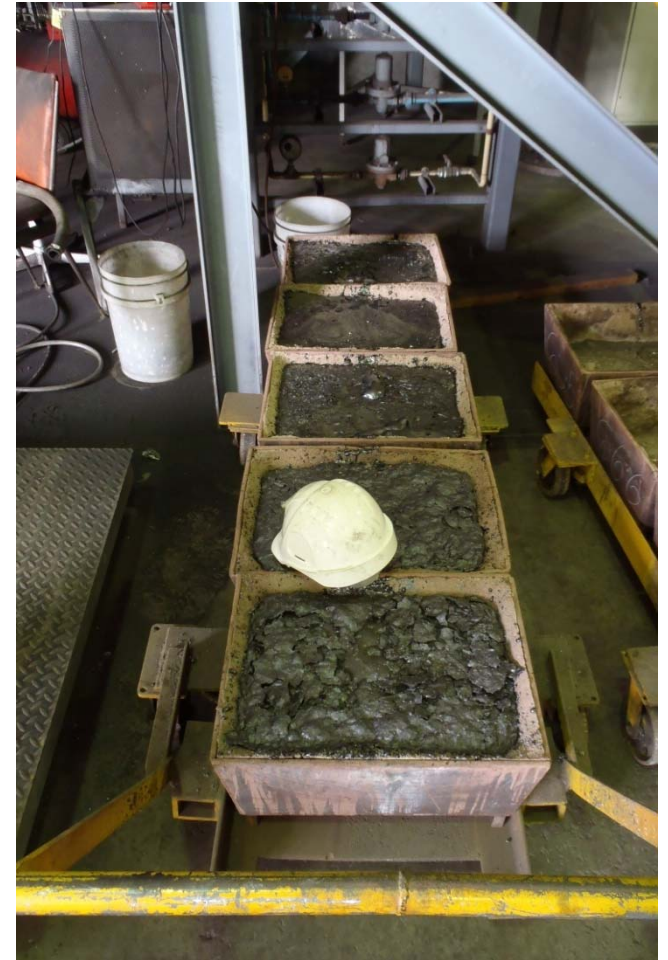
Ausiron process pilot scale hot metal tapping utilising Kulon Progo DRI
