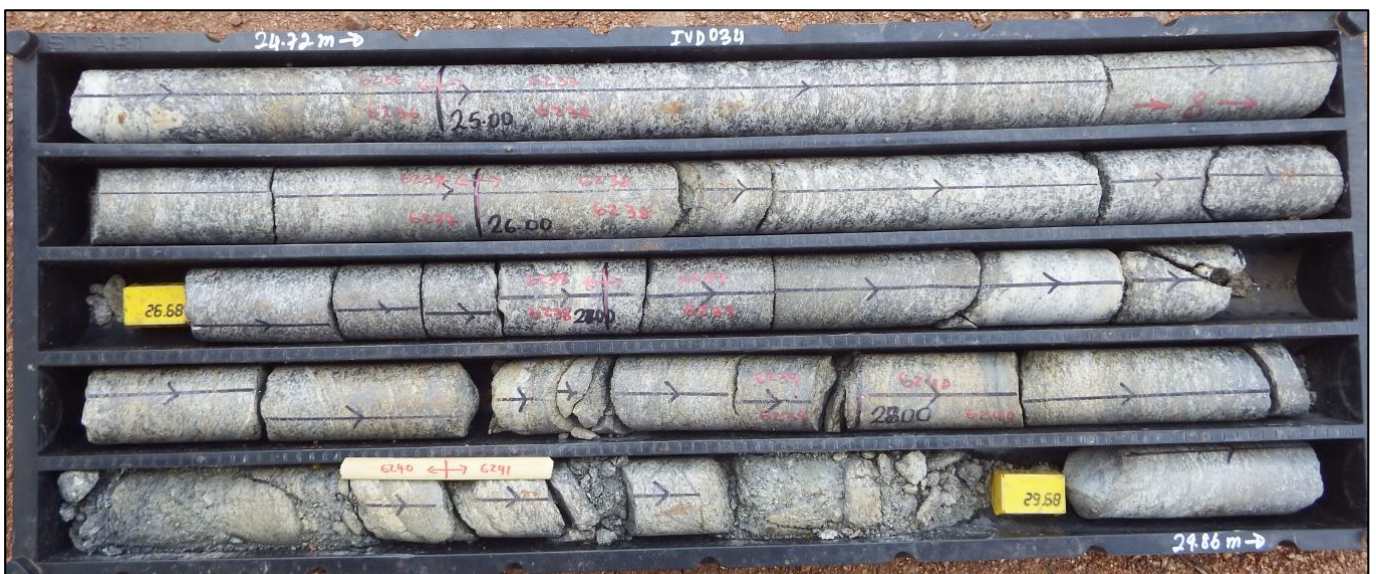
Figure 4: Core samples from T12 IVD034 showing coarse-grained flake graphite in tonalitic gneiss.
