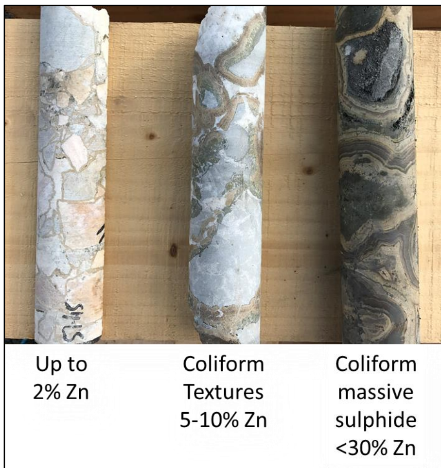
Figure 5, drill core showing various styles of breccia and degrees of mineralisation from the recent drilling program.
