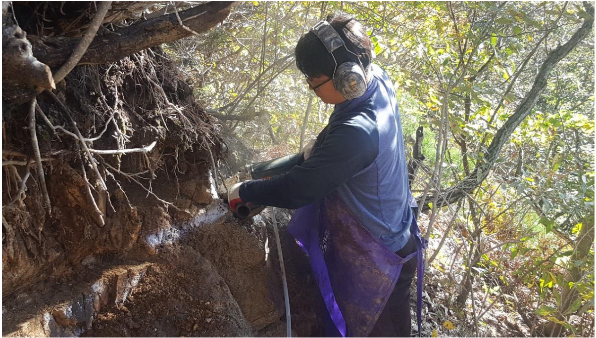
Figure 1: Channel sampling using a rocksaw/angle grinder, Osu Gold Project
