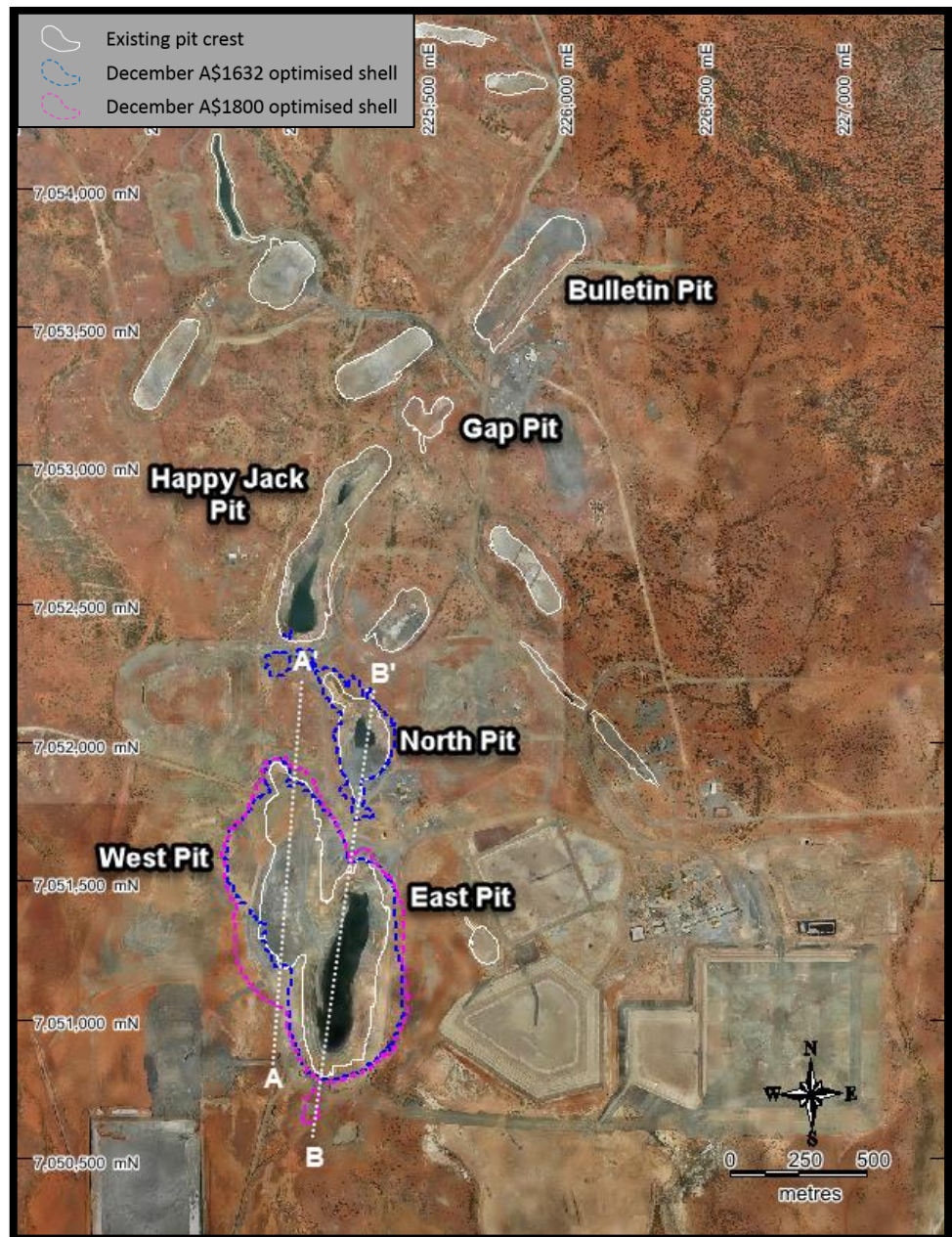
Figure 1 Plan view of Wiluna showing the $1632 and $1800 pit optimisations for the East and West Lodes. Resource estimates are currently being completed for the Happy Jack to Bulletin pits. Long section locations for the West Lode (A-A') and East Lode (B-B') are shown in
