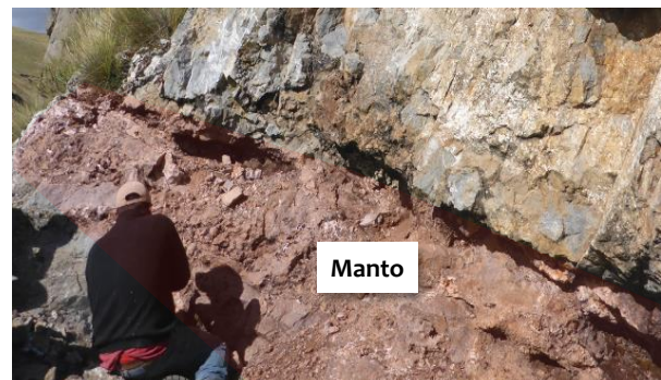
Figure 3: RIGHT Manto horizon (pale red) approximately 1.5m thick dipping into the ground, open in a southern direction. Insert BELOW Galena and sphalerite rich sample taken from the pictured manto horizon.
