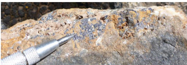
Figure 3: RIGHT Manto horizon (pale red) approximately 1.5m thick dipping into the ground, open in a southern direction. Insert BELOW Galena and sphalerite rich sample taken from the pictured manto horizon.
