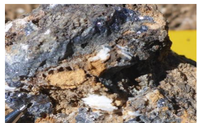
Figure 6: LEFT Photo of vein HV12. It comprises a 1.0m to 1.5m wide vein (pale red) of blebby coarse galena and sphalerite ( Insert BELOW ) and an additional 1.5m wide zone of disseminated galena and sphalerite (pale yellow). Hv12, as well as Hv11, 15 and 16 are believed part of the Callancocha Structure feeder zone.
