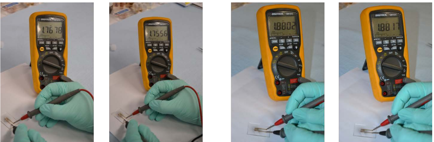
Figure 1: Pristine Graphene resistance 1,700 – 1,900 Ohm
