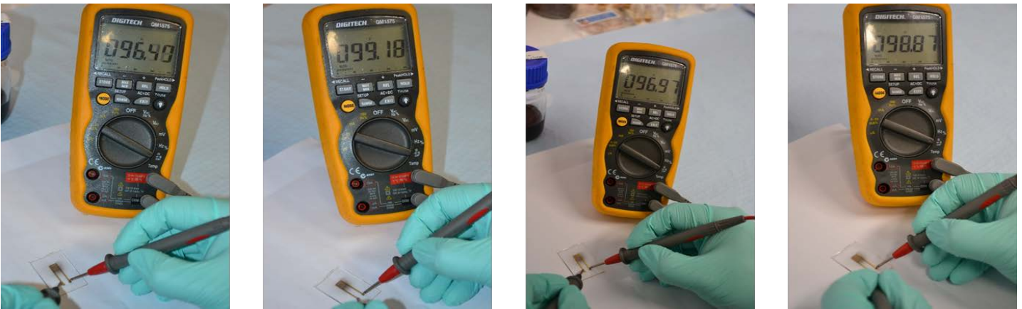
Figure 1: FGR Large area graphene resistance <100 Ohm
