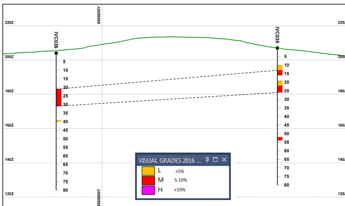
Figure 6: T13 long section looking north, showing visually estimated graphite grades* in holes IVC035 and IVC036. The dashed line polygon is the provisionally interpreted graphitic zone. No vertical exaggeration; downhole depths in metres. Elevations at 20 m intervals.
