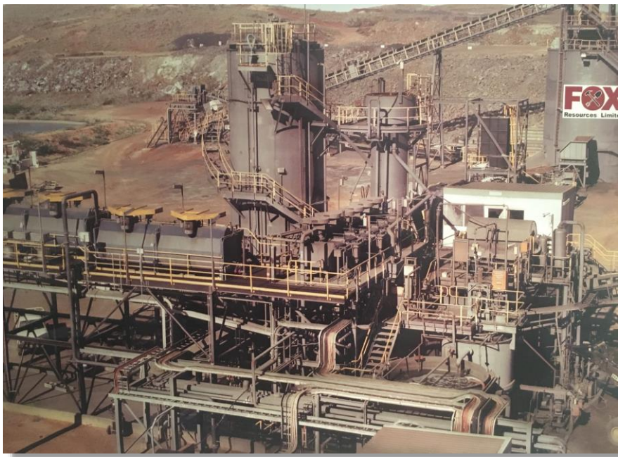
Figure 2b: AGIP Radio Hill Nickel/Copper Operations (Fox 100%) – Radio Hill 425,000 tpa Treatment Plant and flotation circuits.
