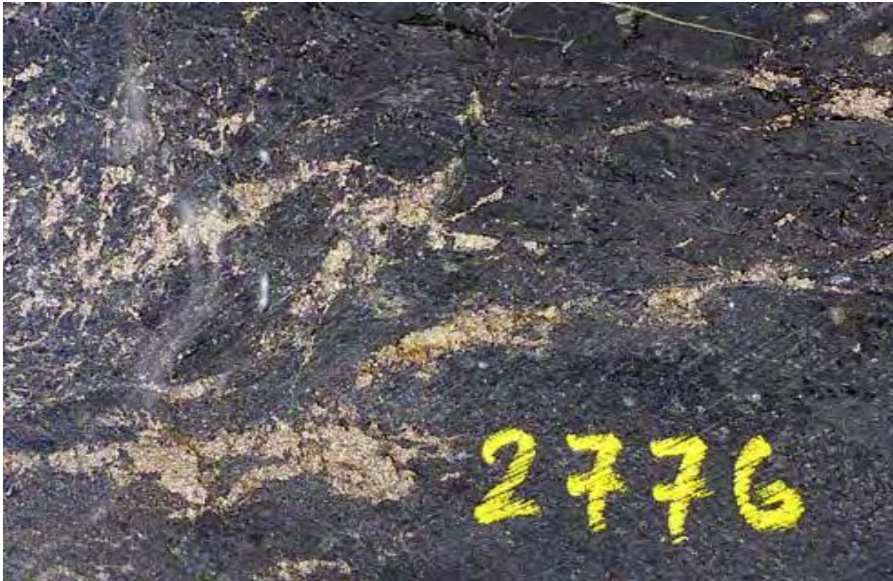
Figure 5. Core from 168.8m in TALDD001 showing graphite with sulphides (pyrrhotite, pyrite) in quartz-muscovite schist. Field of view approximately 3 cm.
