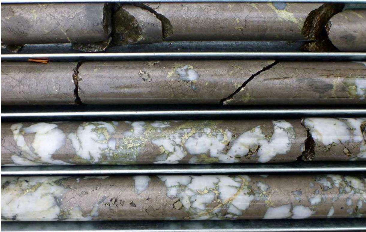
Figure 6. Massive sulphides (pyrrhotite; blebby chalcopyrite) and quartz-chalcopyrite breccia. TALRCDD003 (156-161m)
