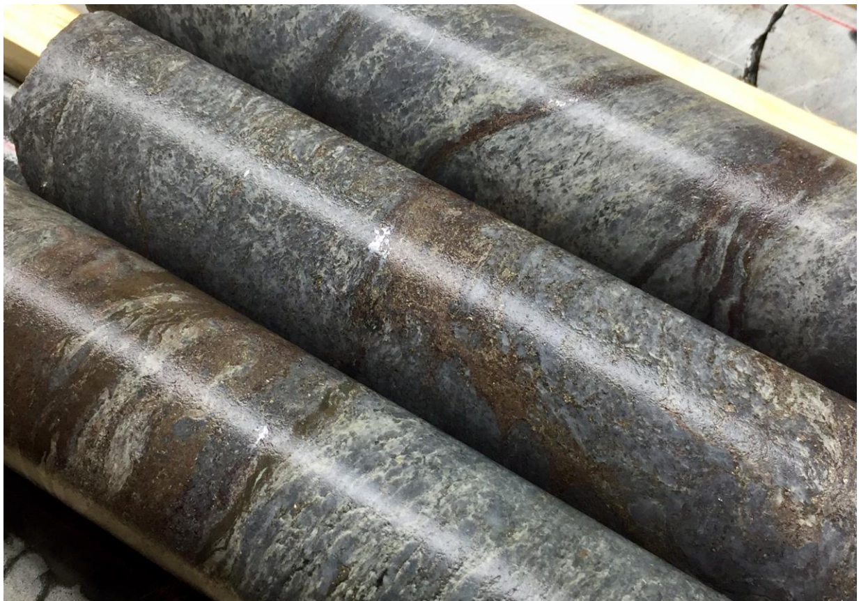
Figure 3. Photograph of stringer sphalerite zones intersected in hole SSVT170004 at the Svan Vit prospect.
