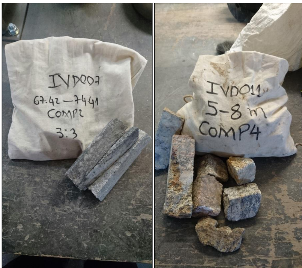
Figure 6: Examples of quarter core samples submitted for metallurgical testing
