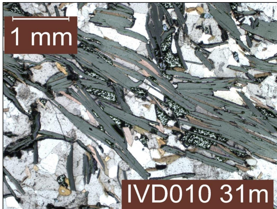
Figure 4: Photomicrograph of graphite (greenish grey) and biotite mica (brown) in a thin section from Composite 5
