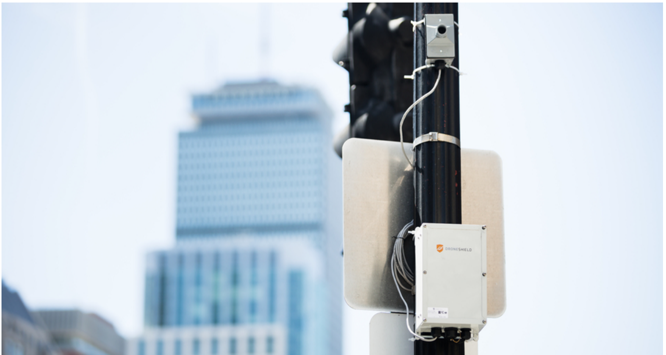
Caption: DroneShield's omnidirectional sensor, of the type purchased by the customer
