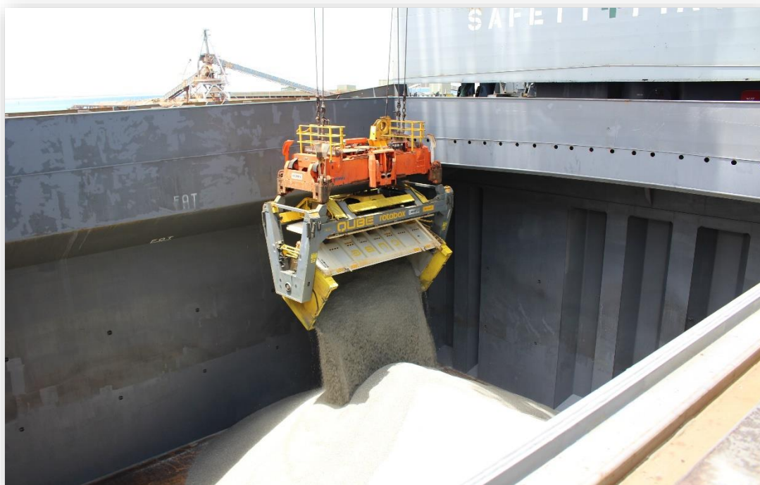
Lithium Concentrate Loading with Qube Rotabox on NY Trader 1
