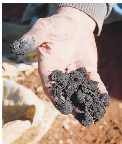
Figure 1 – KNP pyrolusitic ore. This drill sample from 2001 assayed approximately 1% Co and 2% Ni. The cobalt-rich material occurs within the upper part of the cobalt-nickel laterite profile.
