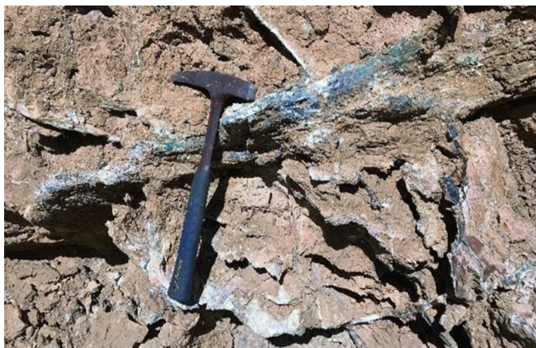
Figure 2 – Run-of-mine KNP siliceous ore. This mine face includes green chrysoprase veining. Chrysoprase material tends to occur within the lower part of the cobalt-nickel laterite profile.
