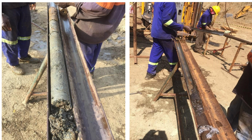
Fig 3. HQ3 core being removed from split inner tube
