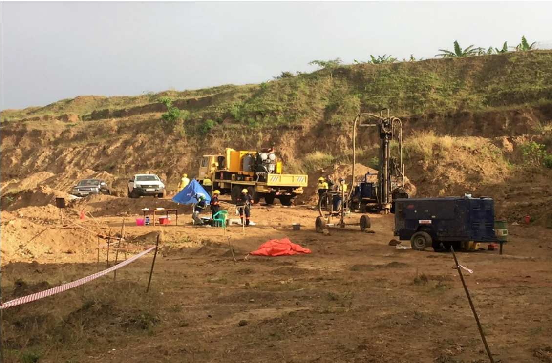
Fig 4. Grade control Aircore Drilling in P1, Hole NGC0012
