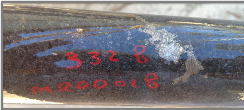
Figure 4; Large magmatic nickel and copper sulphide bleb at 332.8m down hole depth, MRDD018.
