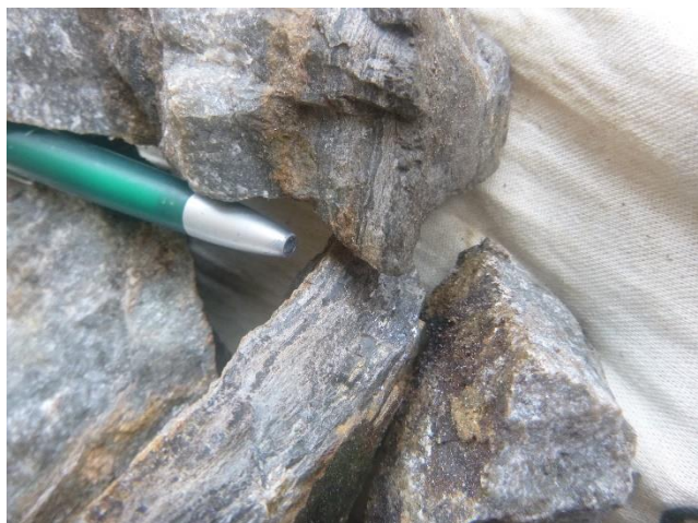
Sample from Niambokamba – Sphalerite bearing mudstone
