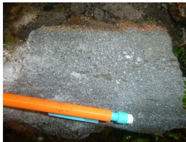
Sample from Niamabimbou – Sphalerite and galena bearing sandstone
