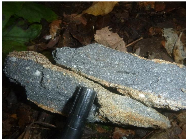
Sample from Dikaki – Sphalerite and galena bearing sandstone
