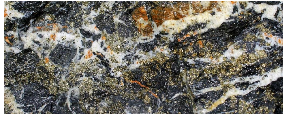
Brecciated shales with quartz fill and disseminated pyrite
