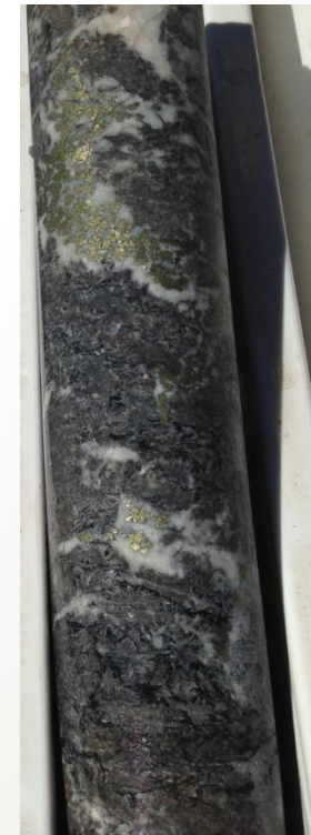
Drill core CCD02, evaporite horizon, disseminated chalcopyrite. Visible ex-gypsum crystals
