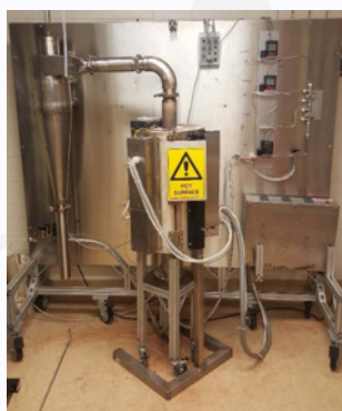
* Hazer's Fluidized Bed Reactor
