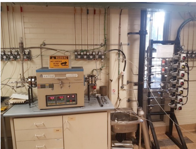
* Hazer's Static Bed Reactor
