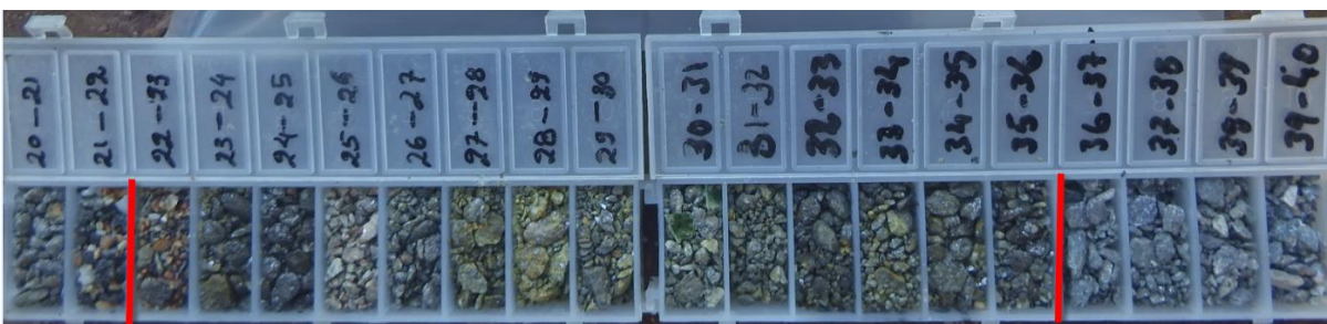
Figure 4: IVC026 RC chips showing graphite mineralisation from 22 to 36 m
