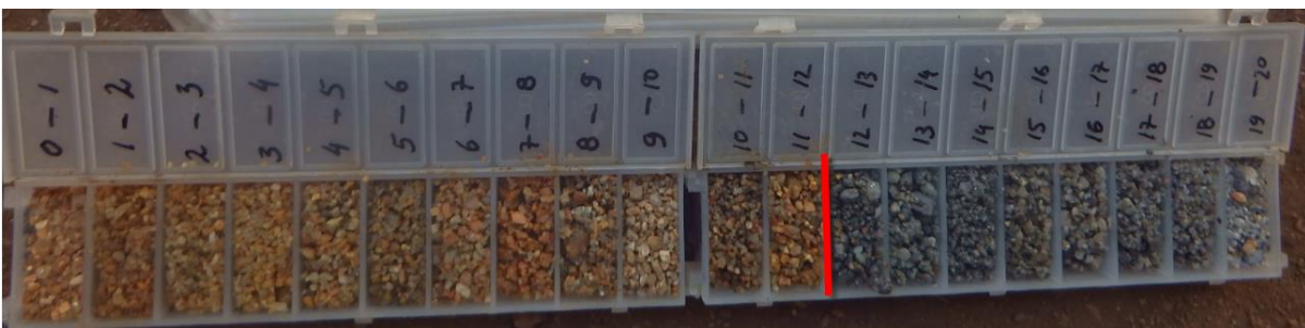
Figure 5: IVC027 RC chips showing graphite mineralisation starting from 12 m.
