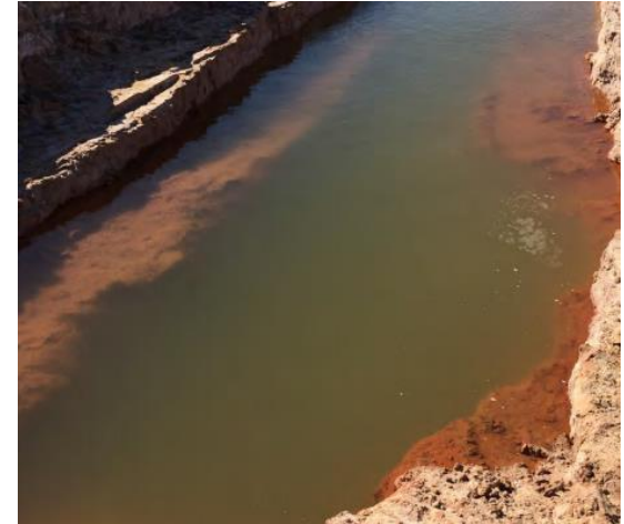
Photo: Potassium brine, Lake Wells 1 Significant evaporation required to generate harvest salt
