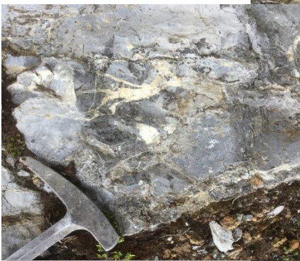
Figure 3: RIGHT The entrance to the Vilcapuquio mine working that returned higher than expected Zn results. Insert BELOW Calcite-veined limestone associated with Zn mineralisation at Vilcapuquio.
