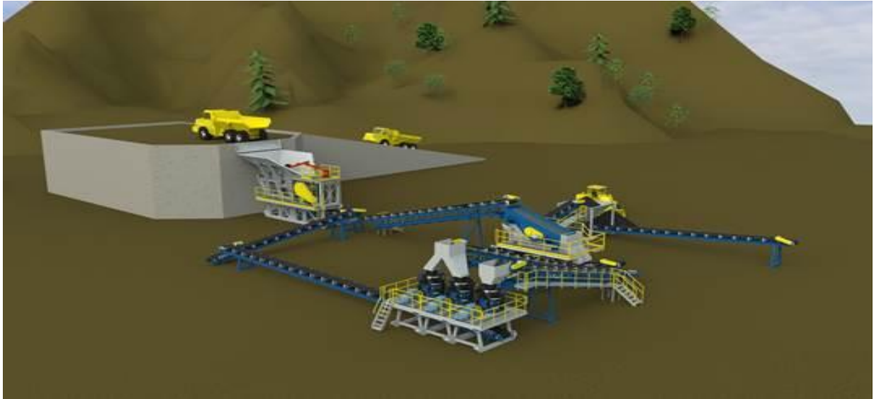
Diagram 1: Sepro Systems 75 tph three stage crushing circuit.
