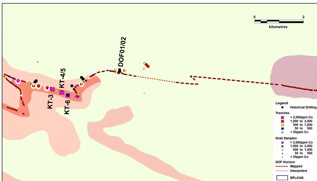
Figure 3. Plan showing area of trenching and drilling within the Opuwo Cobalt Project. CLA verification samples are circled in white.
