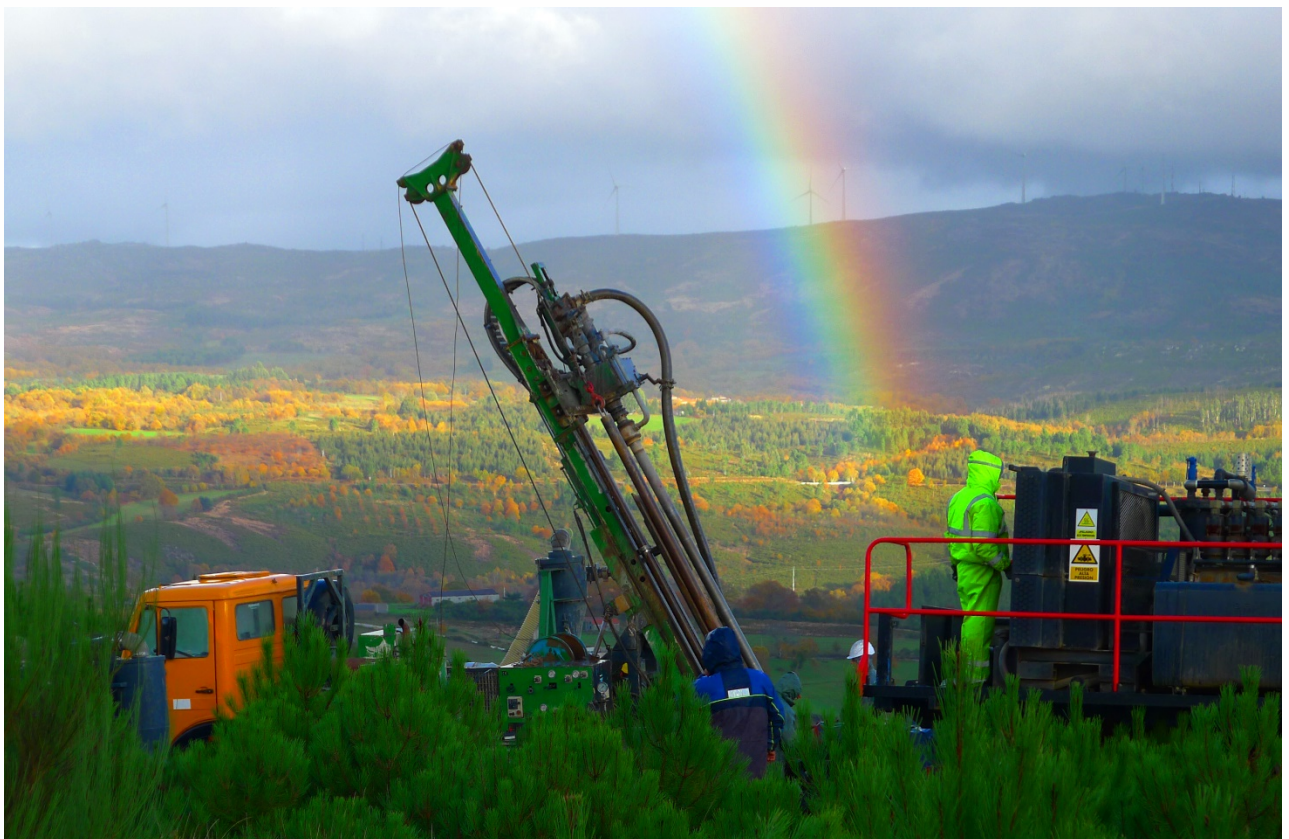
Figure 1: RC drilling at Romano, December 2016 (photo credit: I. Groves)
