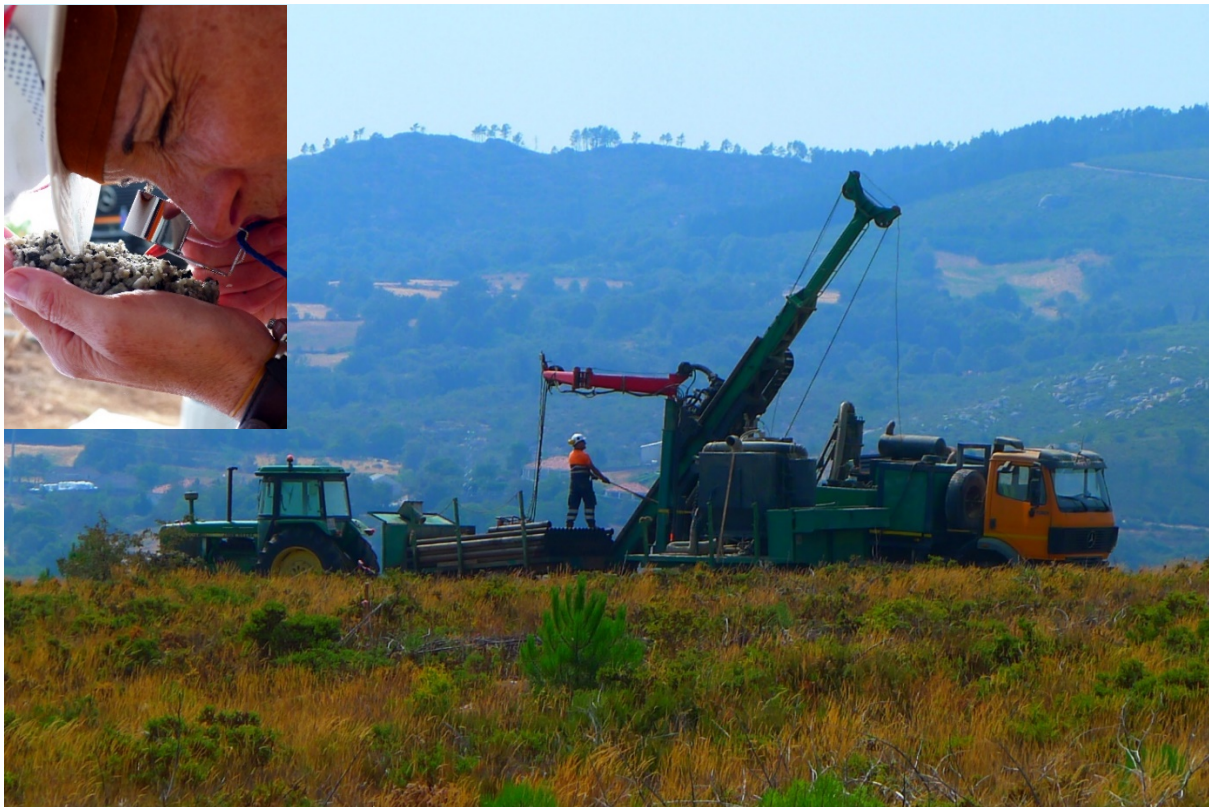
Figure 5: SPI Rig 2 drilling at Sepeda (main photo) and geologist logging RC chips (inset). (photo credit: I. Groves)
