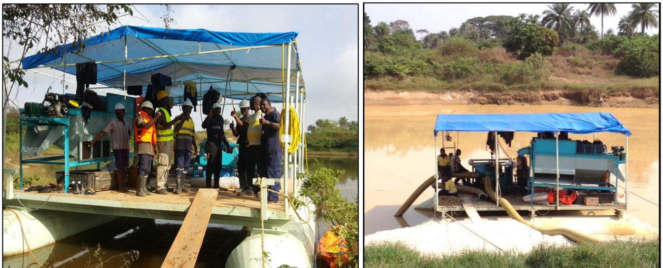
Figure 5. Photo showing one newly-built dredge unit (above), recently deployed on the Komba pit, Sewa River locality, EL 15/2012 (at right).
