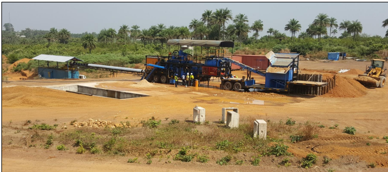
Figure 18. The 10 tph plant is the second to be successfully commissioned by the Company. It will process bulk-samples recovered from the southern licences, and was acquired to circumvent the high-costs and prohibitive distances involved in processing material through the Golu DMS plant.
