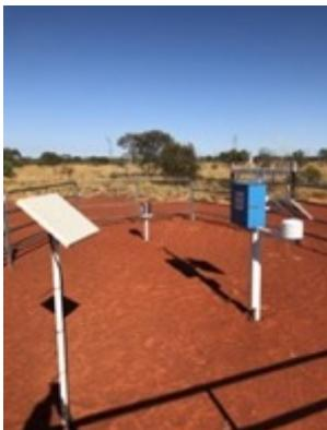
ACP has installed and commissioned a 14 module permanent weather station at the Lake Wells Potash Project. The station is equipped with a remote satellite system, meaning the Company and its consultants are able to collate meteorological data, such as air temperature, barometric pressure and humidity, 24/7. This data will continue to be collected into the life of the project, and feed into the models being built around pond sizing.
