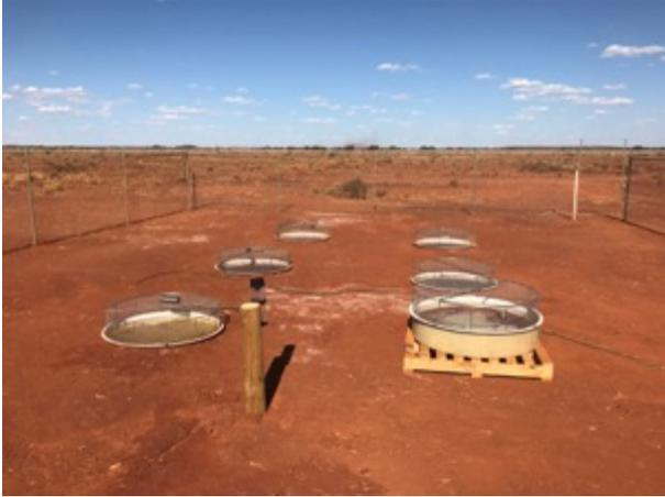
Figure 5: Class A evaporation pan trial
