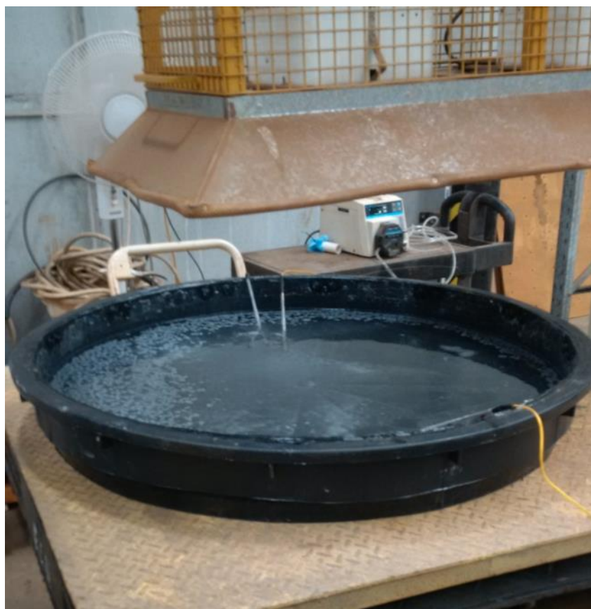
Figure 21 – BV Evaporation Pan Set Up.
