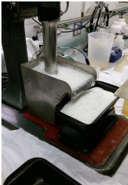
Figure 17: Rougher Flotation Test on Lake Wells Derived Mixed Sulphate Salts
