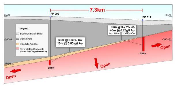
Figure 2: Cross section of previous drilling at Tabac Project
