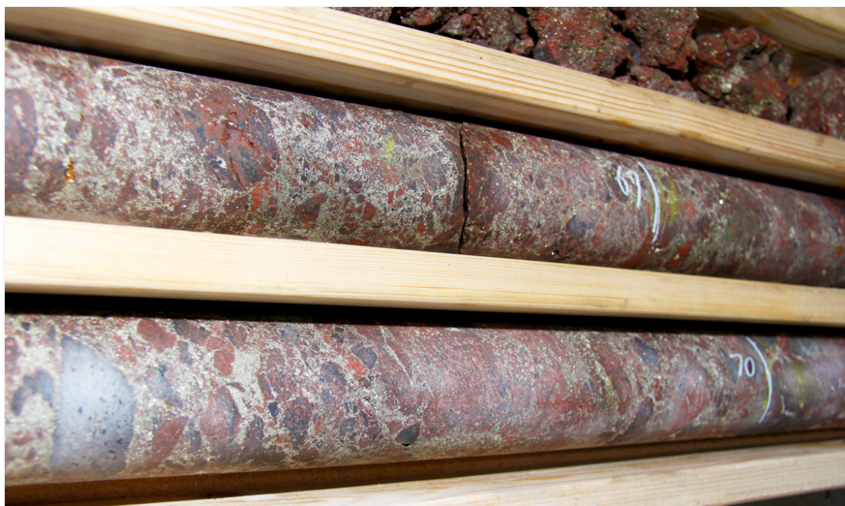
Figure 4 Drillcore from Kiskama showing IOCG style mineralisation (KIS04).
