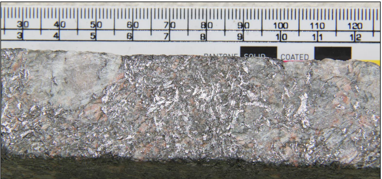
Figure 3: Example of coarse flake graphite in quarter NQ drill core from IVD034 at T16, at approximately 58.5 metres downhole. Sample length 10 cm
