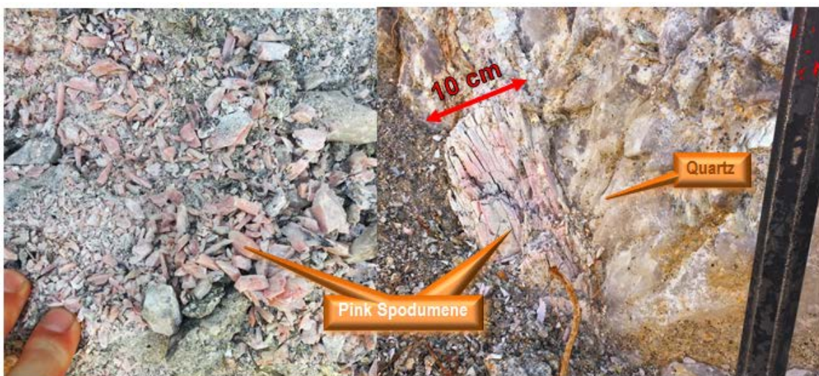
Figure 7 – Examples of pink coloured weathered spodumene in the Maria del Huerto open pit (Intermediate Zone).
