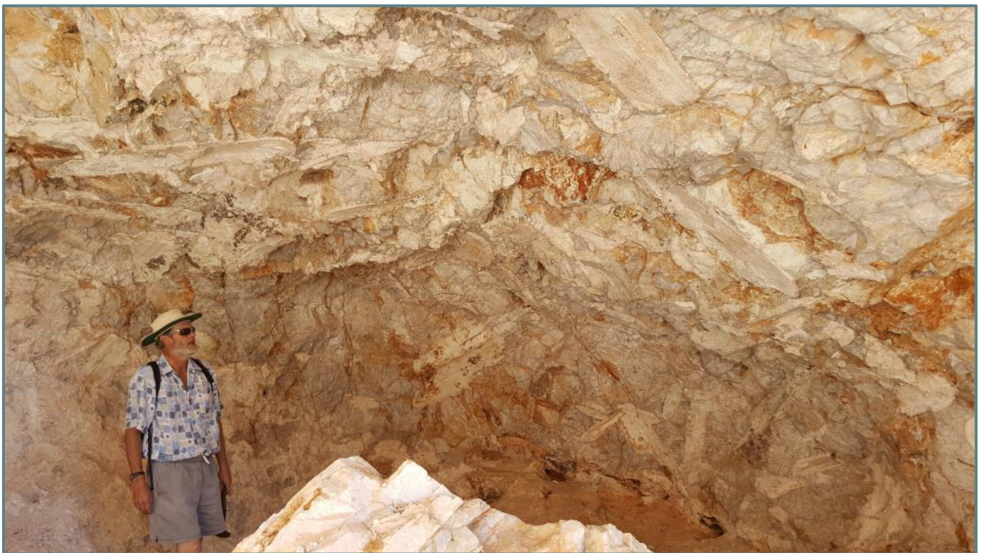
Plate 1 – Exposed mine face showing large Spodumene crystals
