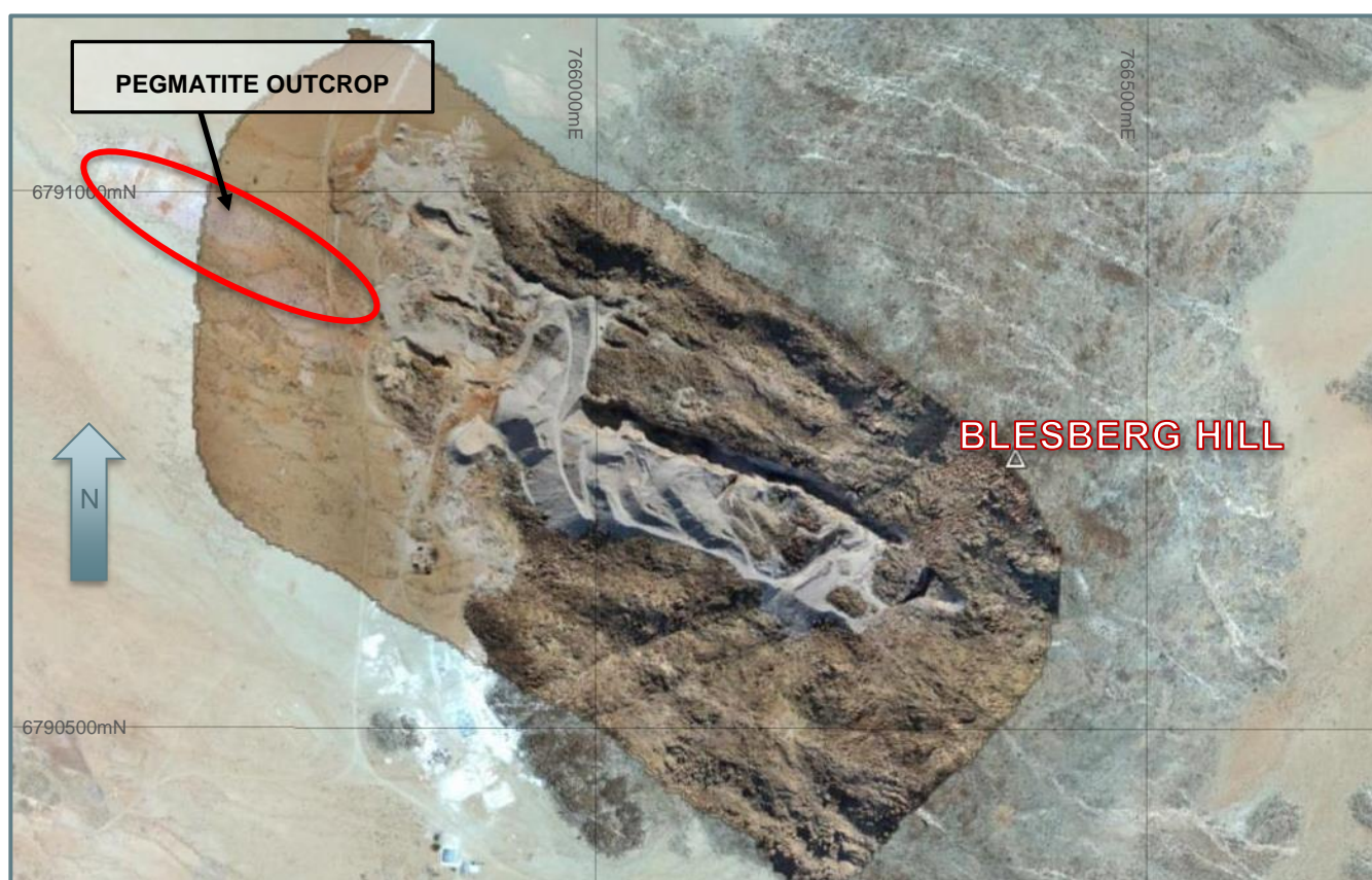
Figure 2 – Blesberg Hill showing old mine workings and numerous pegmatite veins and the mapped pegmatite outcrop interpreted as a minimum 500m extension of the main Noumas1 pegmatite body.
