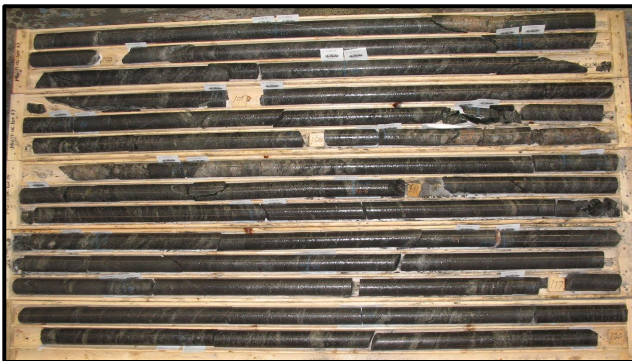
Figure 2. Drill core (MW-16-06) showing substantial graphite mineralisation.
