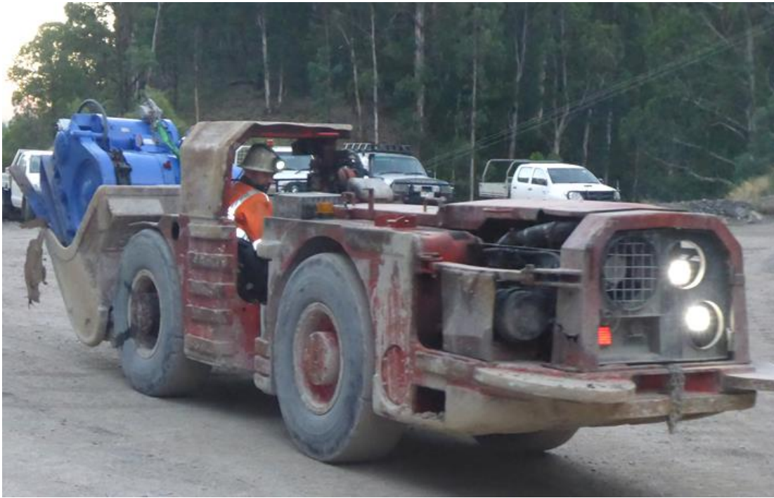
Figure 12. New electrical scraper (Pickrose) for air-leg Stope 1645-8764 being taken underground in the 151 LHD bogger at the A1 Mine.
