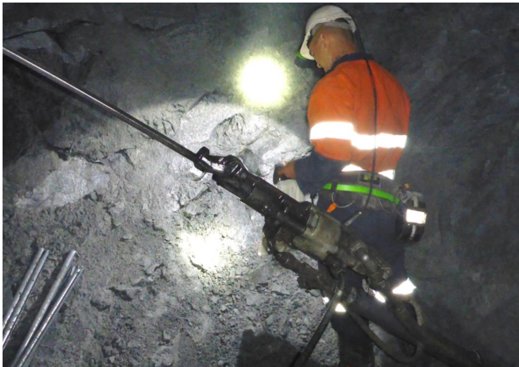
Figure 10. Geologist Russell Price face sampling an air leg development drive at the A1 Mine.
