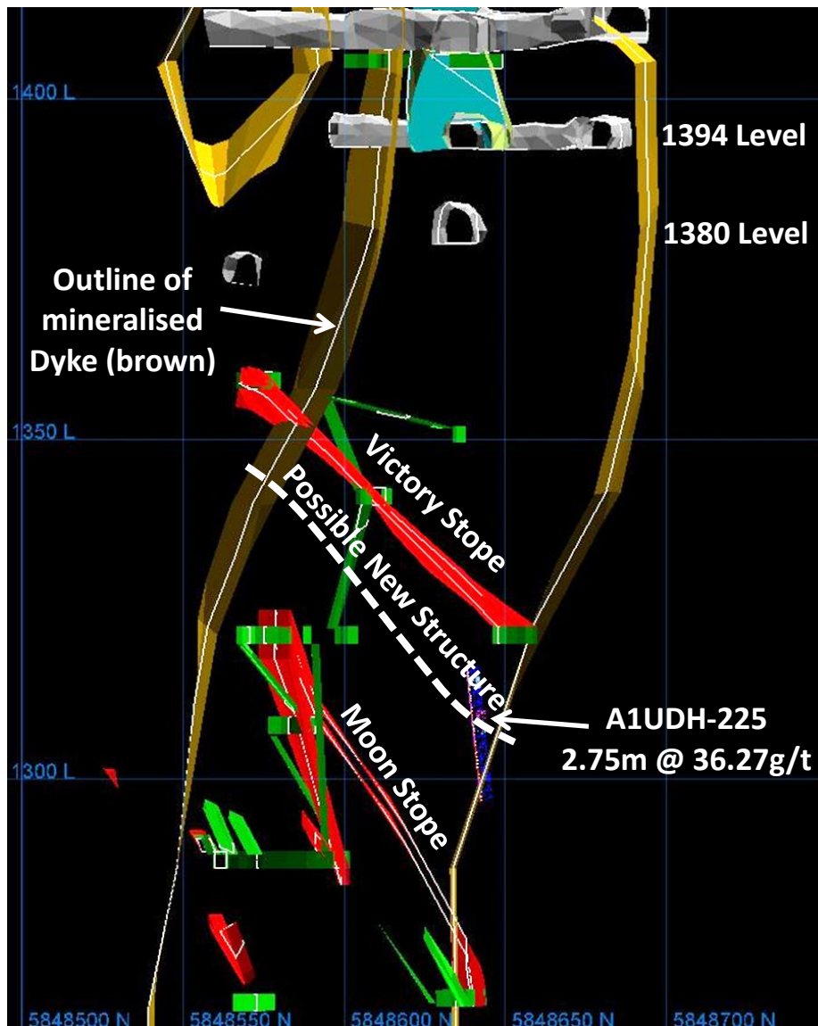
Figure14. Cross Section of the A1 Dyke (outline shown in brown) showing the present working levels, historical development (green) and stoping (red) with location of A1UDH-225.
