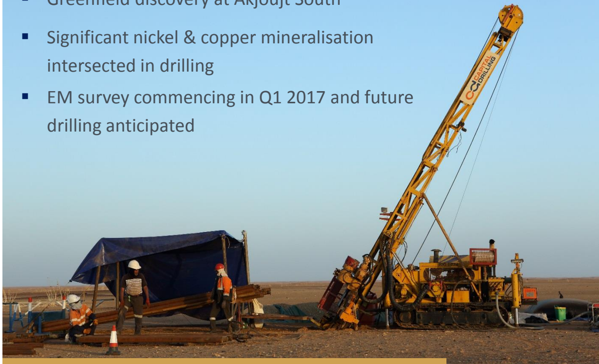
Diamond drill rig at the Akjoujt South Project in Mauritania, March 2016
