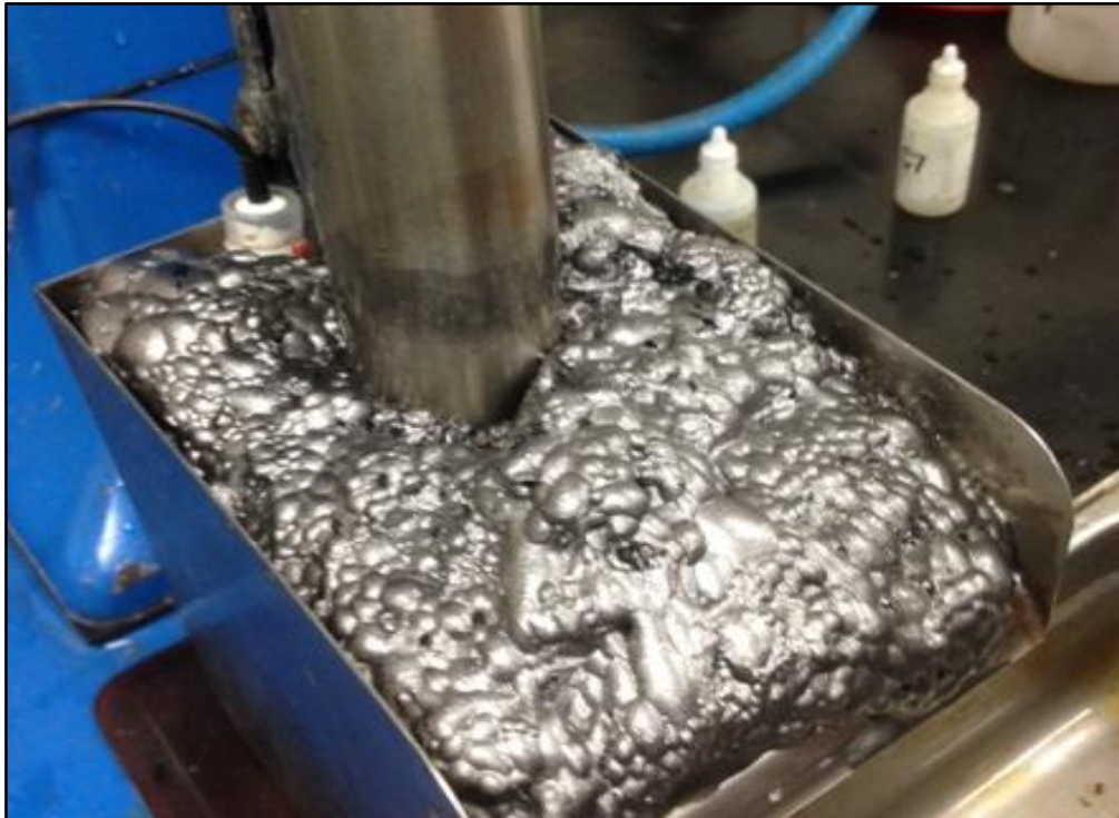
Image: GS03 Weathered Composite Rougher Flotation without Collector; Chemical free production from BAT's graphite
